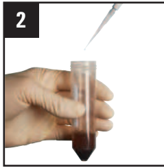
2 Add water and QC spikes if needed and spike with internal standard
