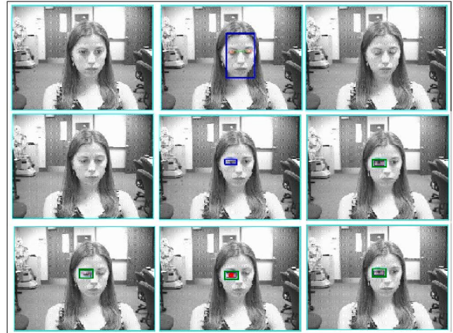
Figure 6: Intermittent frames from a sequence during the motion analysis phase when the template is being found automatically by the user's first several natural blinks. Rectangles around the face indicate that blink-like motion was detected. The small rectangle that appears around the eye three frames later indicates where the open eye template is being selected. The subsequent small rectangles indicate eye tracking. A red circle on top of the eye (third row, second column) indicates that a blink is believed to have just ended.
