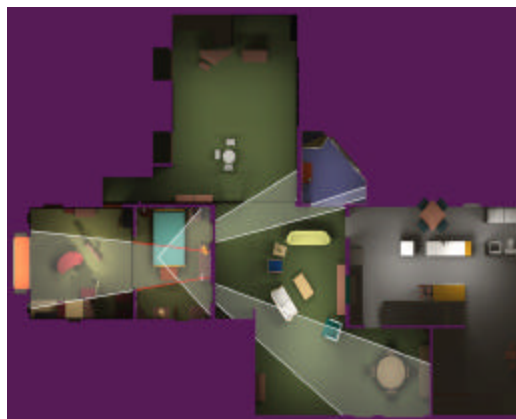
Figure 9. This is an overhead view of the house containing the room in Figure 8. View frustum is clipped against each portal in order to calculate what sectors are visible [1].
