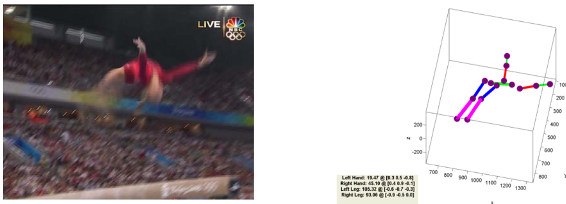
Figure 7. The speed and direction of all four extremities are displayed through this gymnast's balance beam performance.
